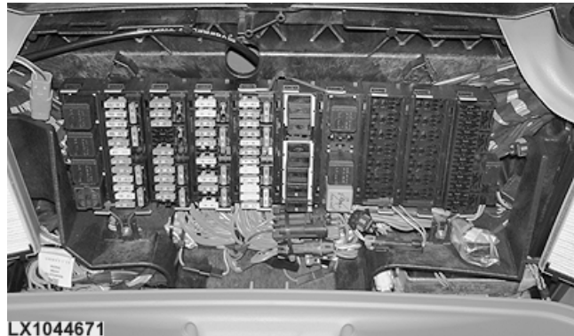
Up to serial number break 2008 (F02 to F05 fuse arrangement)
